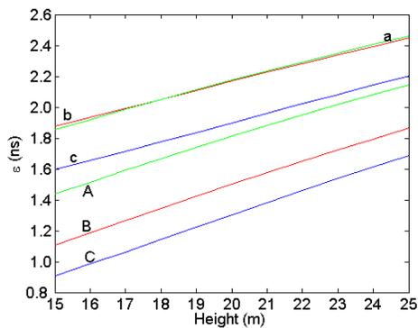
Fig 10. Variation in RMS time delay error,  $\epsilon$ , as a function of height for each of the phases of figure 9.
