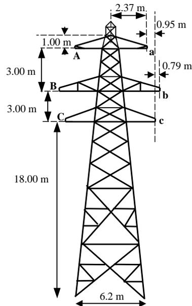
Fig 9. PL4 132 kV overhead double circuit tower with identifying phases.
