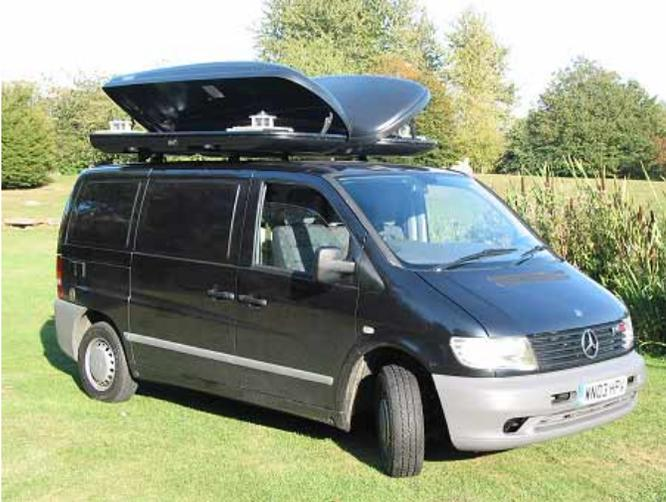
Fig 1. Photograph showing the vehicle mounted antenna array. The sampling equipment is located within the vehicle.
