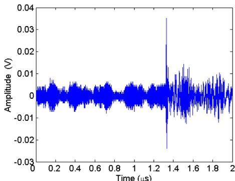
Fig 6. Typical RF impulse recorded from position II.
