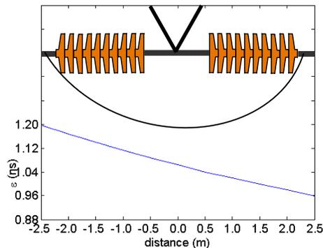
Fig 11. Variation in  $\epsilon$  versus distance along insulator strings. X axis shows offset from centre of cross-arm; van situated in direction of decreasing x.
