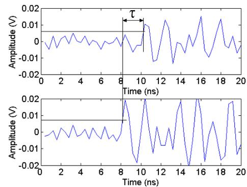
Fig 2. Time delay calculation. Initial wavefront of impulse arrives at the upper trace at 10 ns, and the lower trace at 8 ns.
