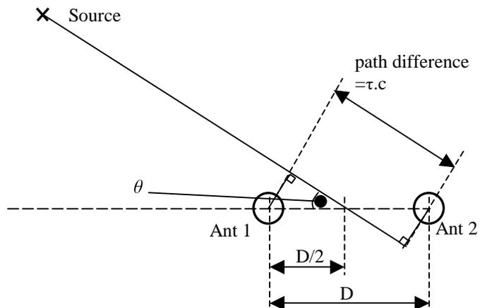
Fig 3. Bearing calculation.
