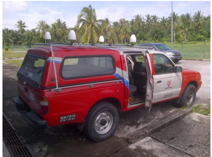
TNB pickup truck fitted with the PDtect4-surveyor hardware prior to a substation survey.
