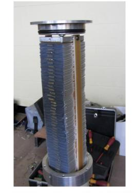
Example grading capacitor (not unit removed from CB)
