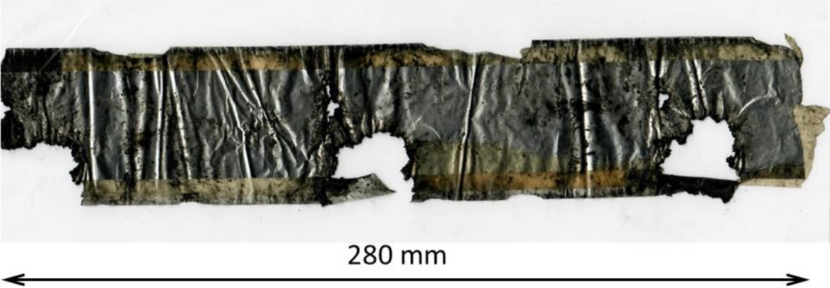
Figure 8 Damage to the foil of an individual capacitor unit.
